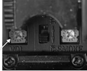
Figure 5: Manual Volume Control
