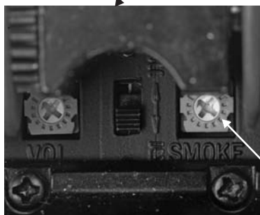
Figure 3: Smoke Unit Control
